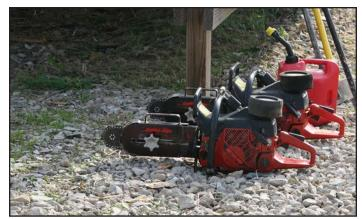
ings are loud and you don't hear that initial chug which indicates to push the choke in. One pull past that chug and you can flood your saw. The most noticeable indication will be a strong smell of gasoline. The fuel to air mixture is too rich in the cylinder to ignite and start the engine.
